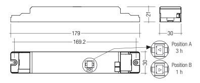
Note: LED Driver supplied with duration link in 3 hours position. Duration link must be set before battery and mains connection.
